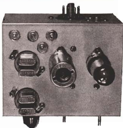
Fig. 6. Top and bottom view photographs of the exciters for 28 and 50 megacycles. Left—the single channel exciter. Right—the four-channel exciter. On both models the 1\frac{1}{2} -inch diameter socket hole for the power connector, J_1 , was punched 1\frac{1}{2} inches down from the chassis deck; and 3 inches in from the oscillator end of the chassis.
