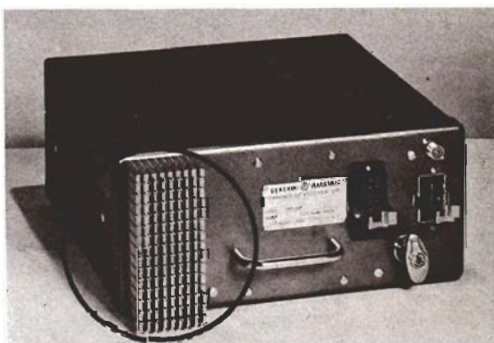
FRONT VIEW of a complete transistor-powered G-E two-way mobile radio with the heat sink for the power transistors on the front panel (inside of circle). Both the power supply chassis and heat sink can be tucked under the dash of an automobile in a space where conventional cube-shaped power supplies would not fit.
