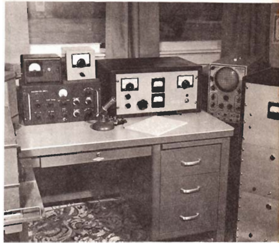
COMPLETE STATION at K2IOW with the Compact Triode Kilowatt at the right side of the operating desk. Other equipment includes an NC-240D receiver and speaker (extreme left); the 6L6-GC exciter which drives the 810 final; indicator for SWR bridge and High-C Bandswitching VFO atop the exciter; 5-inch 'scope for monitoring; and a 3-foot-high rack cabinet containing (top to bottom) class B GL-805 plate modulator, high voltage supply for the modulator, and a 2,000-volt DC supply for the 810 final.
