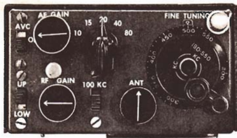
PANEL VIEW PHOTO of the bandswitching converter. Only the controls marked "RF GAIN," "ANT.," and "80-40-20-15-10" (the bandswitch) actually control circuits in the converter.
