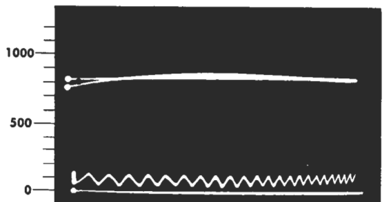
FIG. 8 Load removed ( C_a=0; C_b=90 mfd)
