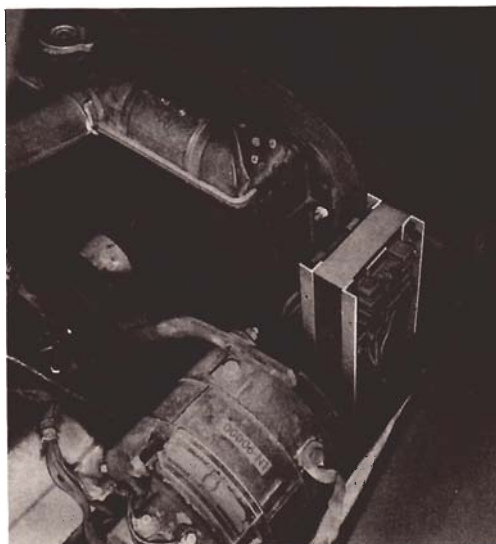
ENGINE COMPARTMENT VIEW of W8DLD's station wagon, showing Lece-Neville alternator in foreground and 3-phase distribution transformer mounted just ahead of it next to radiator.
