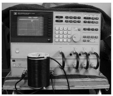
Figure 9 — HP3577A with an HP35677A S-parameter test box.
