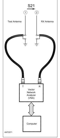
Figure 2 — This diagram shows the vector network analyzer approach for measuring antenna performance.
