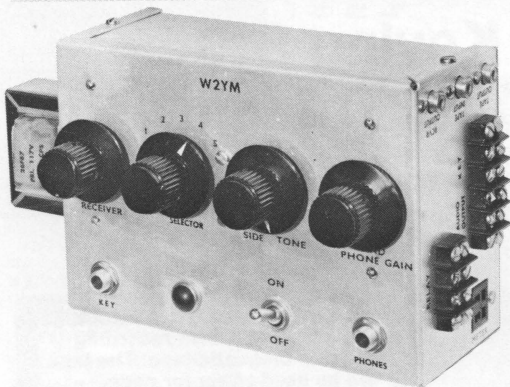
Figure 1: The W2YM magnetic-tape keyer control, or "Keyer." All components are contained within a 7-by-5-by-3-inch minibox with the exception of the power transformer.
