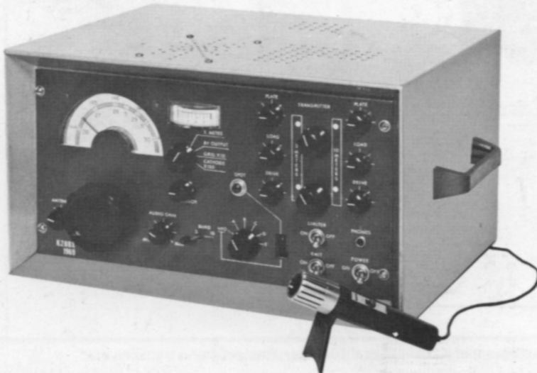
Figure 1: View of completed K2BBX transceiver with RCA HK-99 Star-maker microphone. Unit measures 8 inches in height, 14 inches in width, and 10 inches in depth, and has a carrying handle for easy portability.
